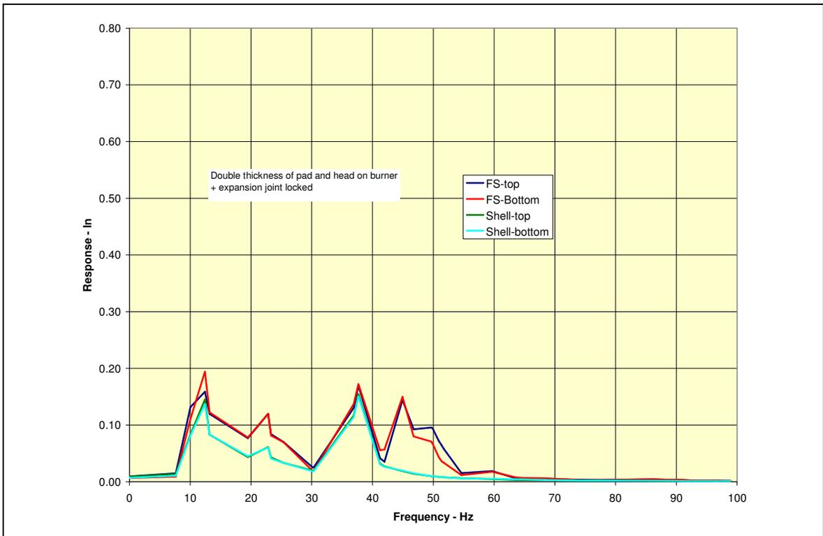
Figure 12 – Displacement with extended and thickened pad and thickened head – joint locked
