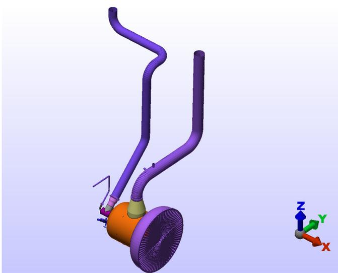
Figure 1 – Image of model of burner and piping
