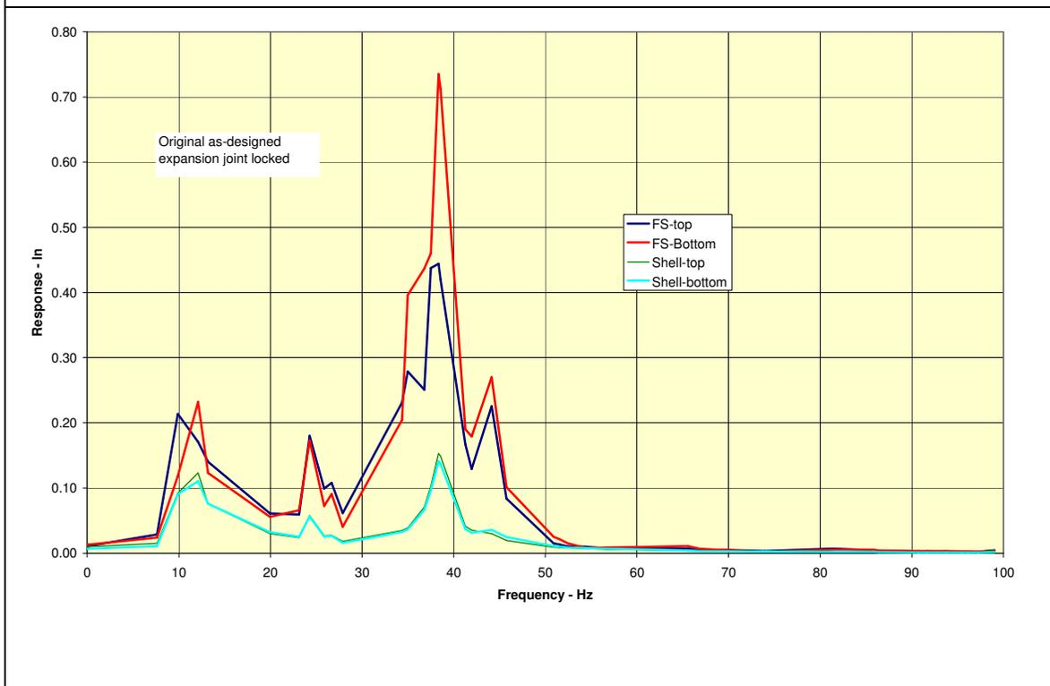
Figure 4 – Displacement for original as-designed system – expansion joint locked
