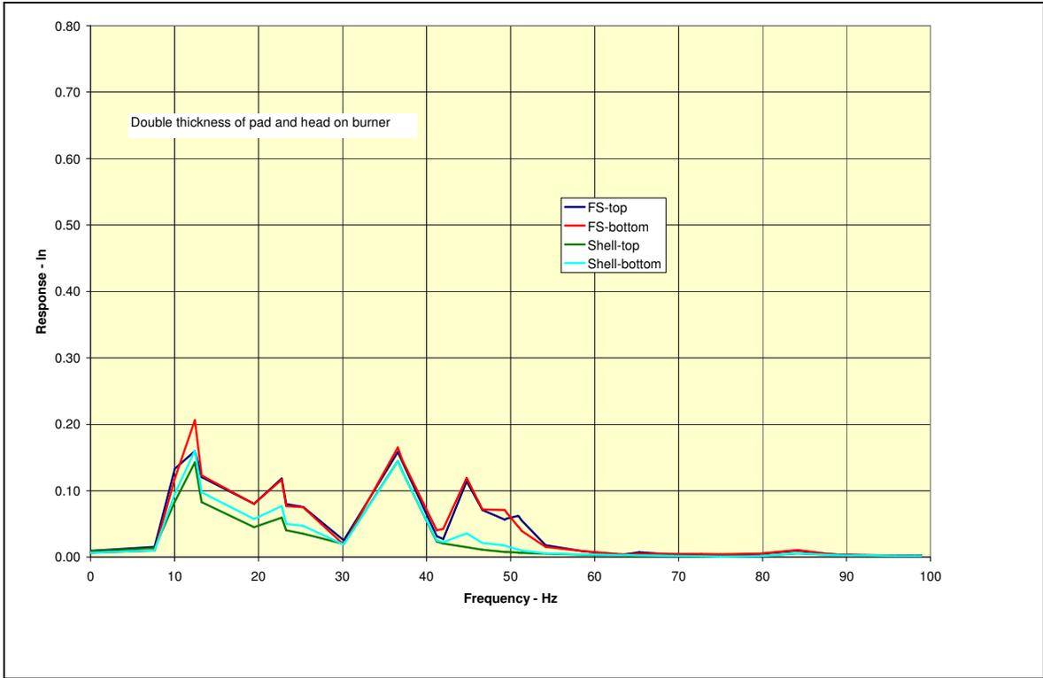
Figure 11 – Displacement with extended and thickened pad and thickened head
