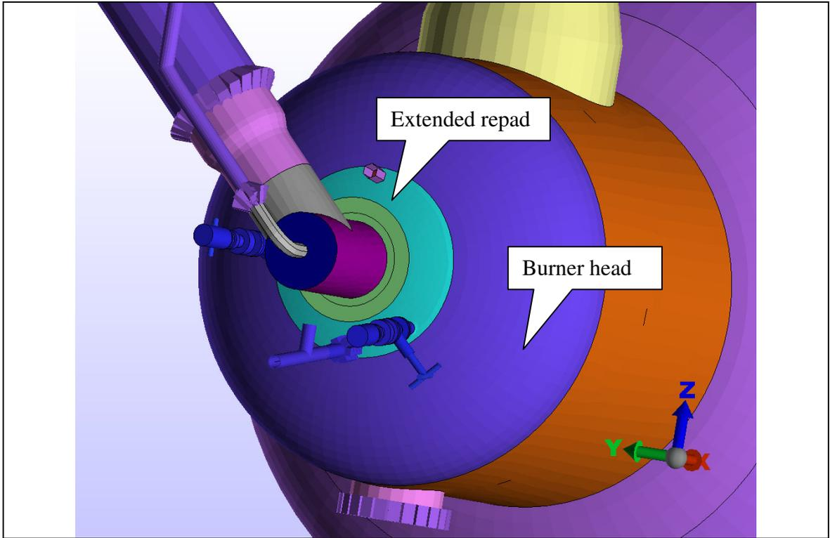
Figure 9 – Extended repad and burner head locations
