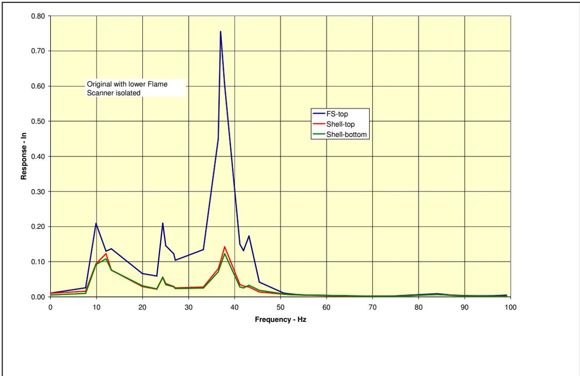
Figure 5 – Displacement for original as-designed system with bottom FS removed
