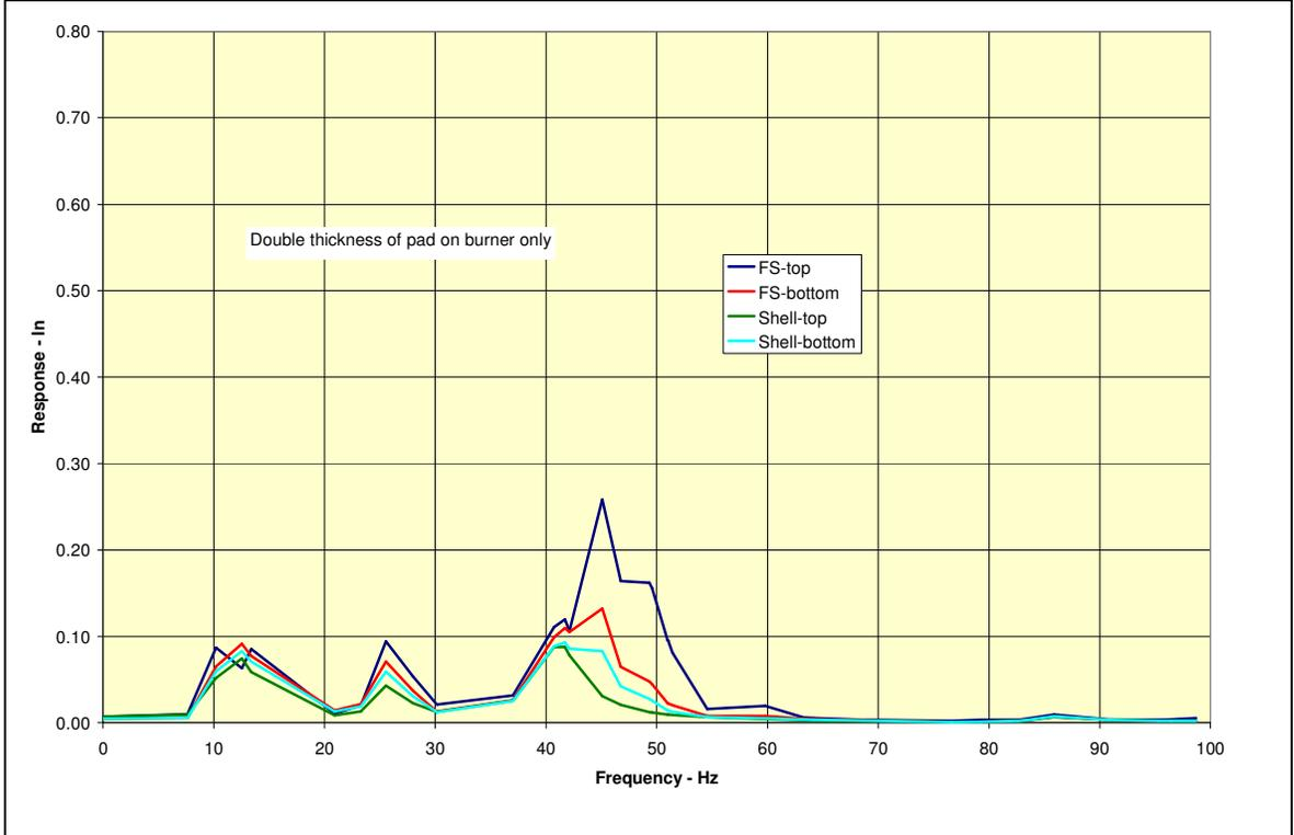
Figure 10 – Displacement with extended and thickened pad
