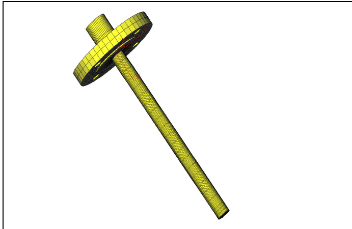
Figure 2 – Basic thermowell model
