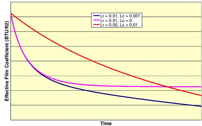
**FIGURE 10 – EFFECTIVE FILM COEFFICIENT VERSUS TIME**
