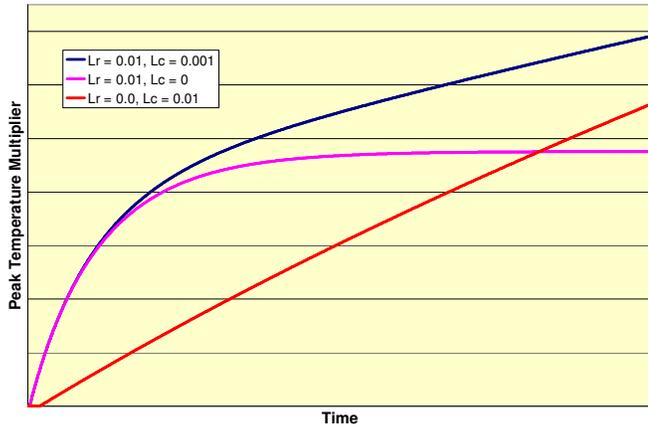
**FIGURE 12 – TEMPERATURE MULTIPLIER VERSUS TIME FOR ASSUMED FOULING REGIMES**
