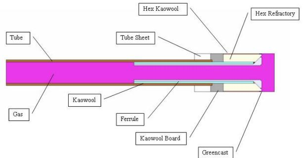
**FIGURE 3 – DOMAINS USED FOR PROCESS SIDE CFD ANALYSIS**
