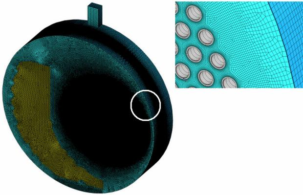
**FIGURE 14 – 3D MODEL USED FOR SHELL-SIDE CFD ANALYSIS**
