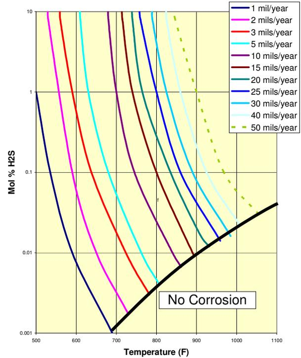
**FIGURE 1 – AUTHORS’ PROPOSED SULFIDATION CORROSION CURVE FOR CARBON STEEL**
